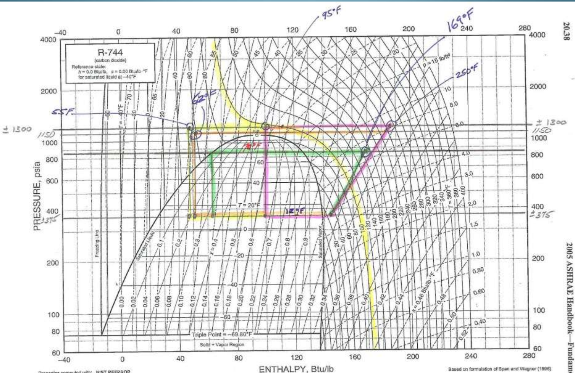
Fig. 18 Pressure-Enthalpy Diagram for Refrigerant 744 (Carbon Dioxide)
